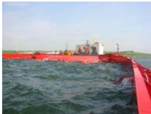
Figure: 5 Wave Dragon Overtopping Device [13]
